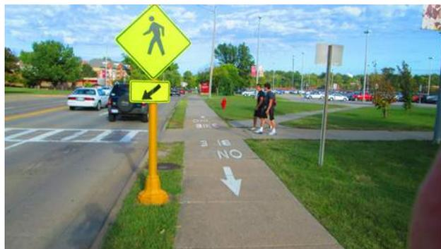
Replace existing continuous flash beacon with RRFB. Widen existing sidewalk to 10' sidepath.
