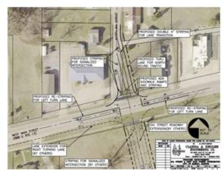
Figure 5.23 - Plan view of proposed 5th Street extension project at reconfigured intersection with W Main Street
