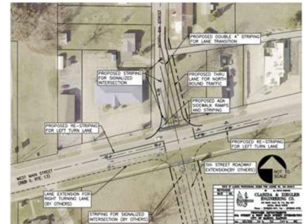
Figure 5.23 - Plan view of proposed 5th Street extension project at reconfigured intersection with W Main Street
