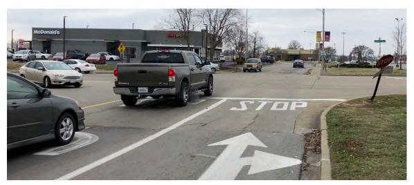
• Southbound Giant City Road. The two-lane approach has a shared through-right lane and a shared through-left lane. The shared through left turn lane is offset from the opposing through movement by 9 feet – the width of the painted median. The approach is stop controlled. Note the proximity of the signalized intersection at IL Route 13. See Photo 3.
