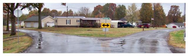
The Skyline Road and Crenshaw Road intersection has 3-legs and is configured as a T-intersection. The stem of the T-intersection (Skyline Road) is stop controlled whereas the Crenshaw Road approaches have right of way. The posted speed limit on Skyline Road is 50 MPH.
