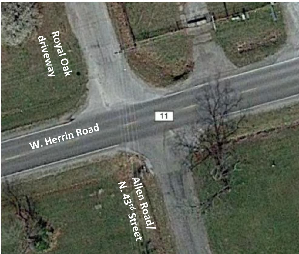
W. Herrin Road is a 2-lane roadway having lane widths of 12 feet and paved shoulders of 4 feet. Passing is permitted within the study area with a 4" yellow skip dash marking. W. Herrin Road was resurfaced in August 2013.
