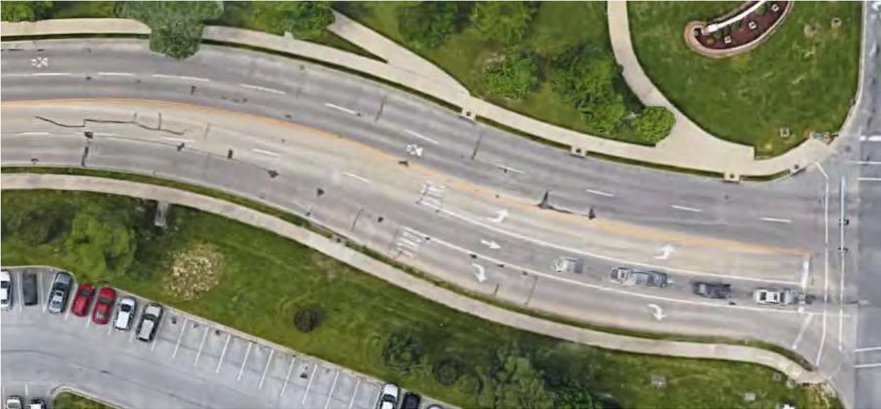
The sight distance on the westbound approach is restricted by the alignment of the opposing traffic (see **Figure 3**). The available intersection sight distance (ISD) of approaching vehicles is reduced to 160 feet. The ISD for a posted speed of 30 MPH is 290 feet for a single unit delivery truck.
