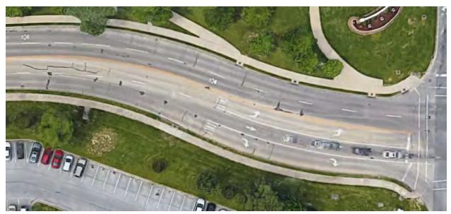
FIGURE 2: HORIZONTAL CURVES AND LANE CONFIGURATION (GRAND AVE)
