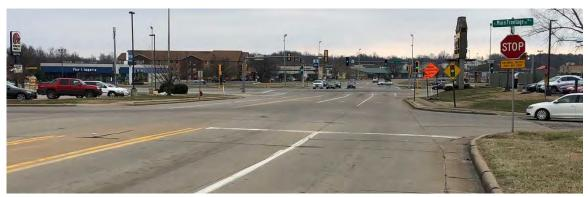
• Northbound Giant City Road. The two-lane approach has a shared through-right lane and a shared through-left lane. The approach has right of way (no stop control). See Photo 4.
