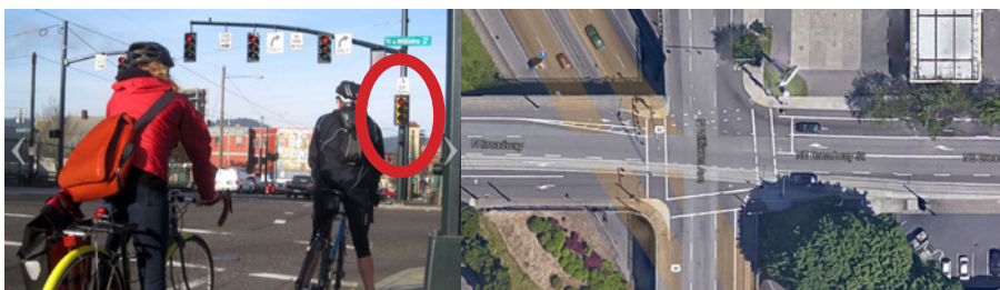
Left: Photo and aerial view example of bike signal at dual right turn intersection. The bike sign allows a bicyclist to move through the intersection prior to vehicles.
